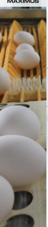
The Egg Flow regulates and adapts the speed of the conveyor belts to ensure both safe and quicker transport of the eggs from the nest or cage to the egg packer, in perfect synchronization. This functionality makes for fewer dirty and cracked eggs, and quicker transport guarantees a quicker temperature control of the egg. In terms of labor management, it helps save time and improves the workstation ergonomics.
